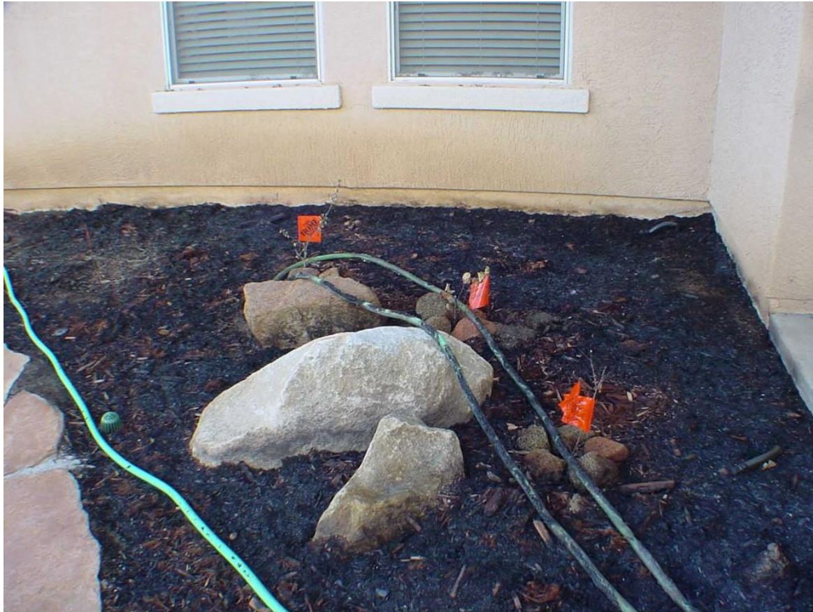
Figure 7: This is an example of how the consolidated shredded redwood bark actually behaves in fires. With overhead irrigation it mats down to less than an inch thick and adheres to the soil. In this case, you can clearly see the scorch marks at the base of the house - <2". Also note the un-melted marker flags that were placed BEFORE the fire (except the one that is partially melted due to the burning hose!). Also note the drain grate next to the flagstone that is unaffected
